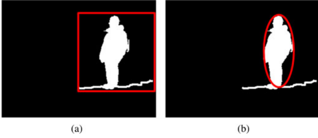
Fig. 5. Comparison of (a) rectangular fitting and (b) ellipse fitting. A line underneath the human's feet is obtained due to the poor segmentation.
