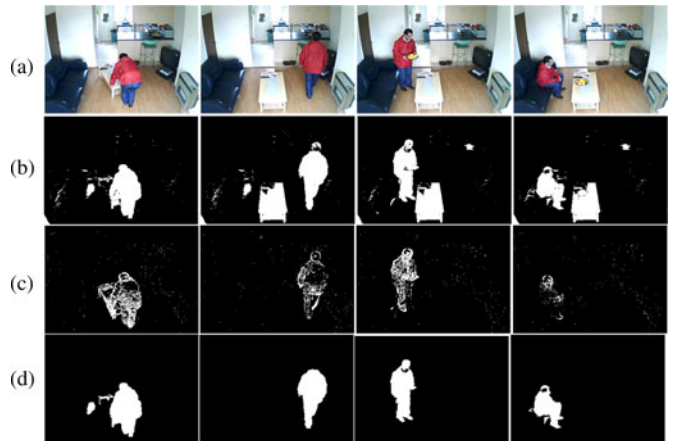
Fig. 11. Background subtraction results for moving furniture. Line (a) shows original frames of a person moving the table and fruit plate. Codebook background subtraction results are shown in line (b). Line (c) shows the frame differencing results which indicate active pixels. From the frame differencing results and blob operations, improved background subtraction results are obtained in line (d).
